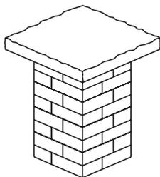
Antique Hampton Wall easily creates columns and pillars with a single block. Run electrical conduit up through the center to create elegant light standards. Top with a Valentia Pier Cap for a natural finishing touch.
